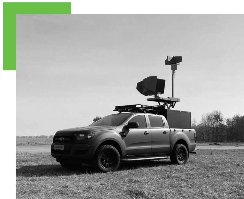
A Ukrainian Bukovel-AD System to detect and jam drones, photo: Ukrspetsexport
