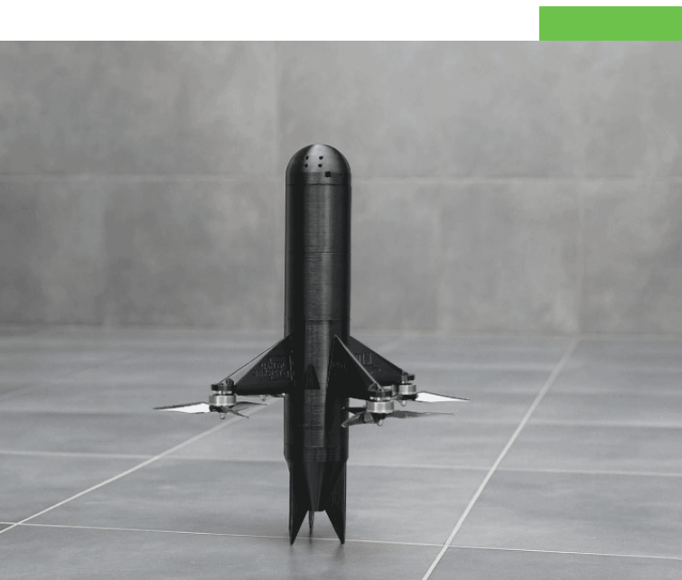
High-speed ODIN Win_Hit FPV interceptor drone in vertical launch configuration, designed to intercept enemy drones in flight, ↗ Militarnyi, 16.7.2025
